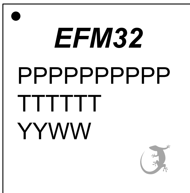
Figure 11.3. TQFP64 Package Marking
