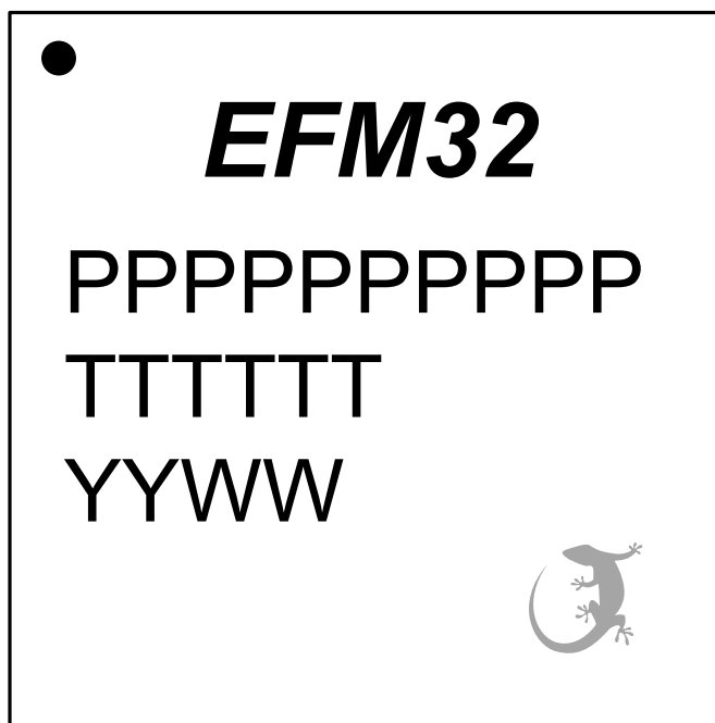
Figure 8.3. BGA120 Package Marking
