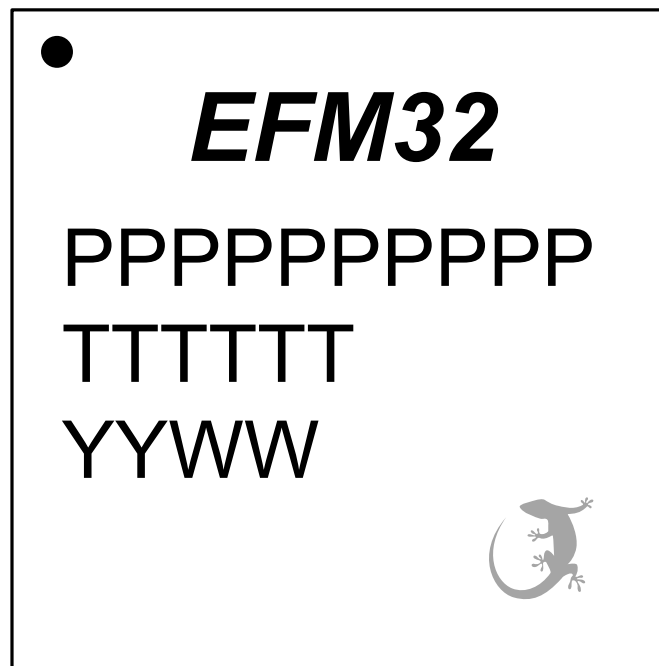
Figure 11.3. TQFP64 Package Marking
