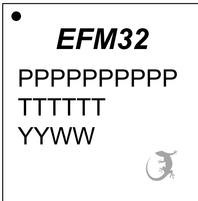
Figure 11.3. TQFP64 Package Marking
