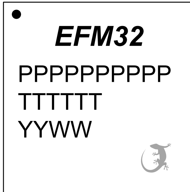
Figure 6.3. BGA192 Package Marking
