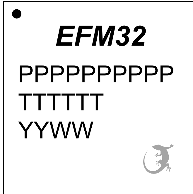
Figure 7.3. BGA152 Package Marking
