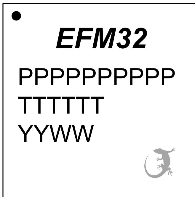
Figure 8.3. BGA120 Package Marking
