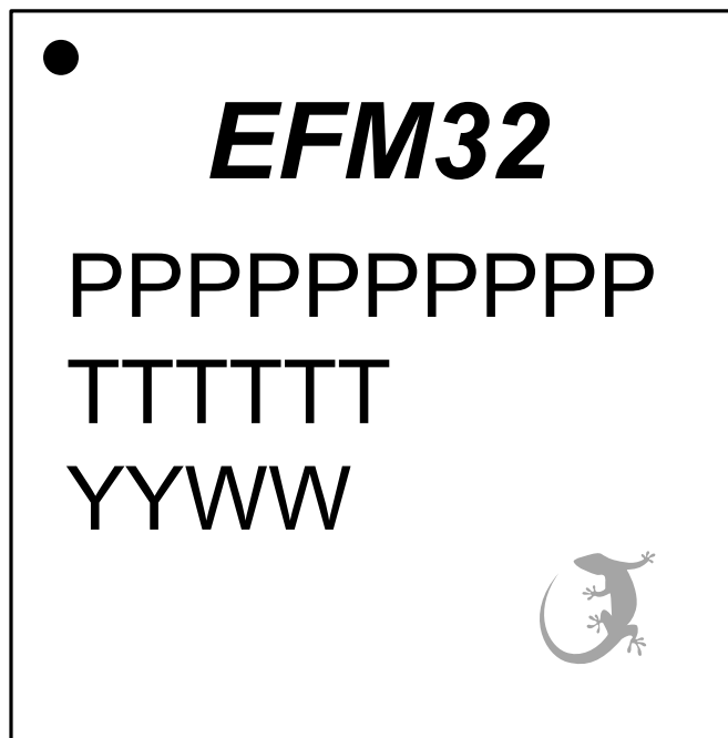
Figure 10.3. TQFP100 Package Marking
