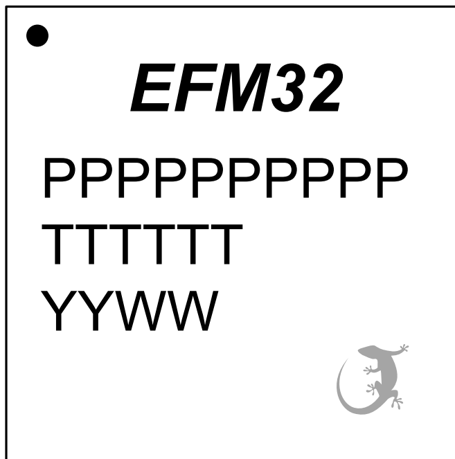
Figure 7.3. BGA152 Package Marking
