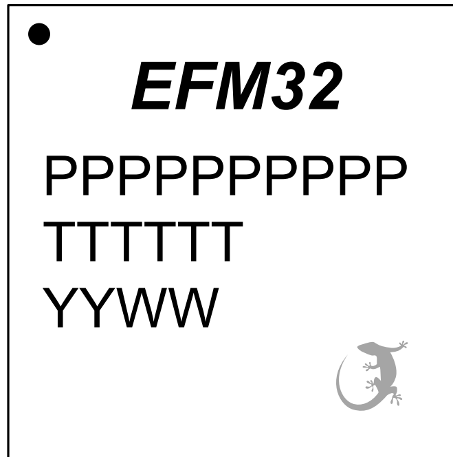
Figure 8.3. BGA120 Package Marking
