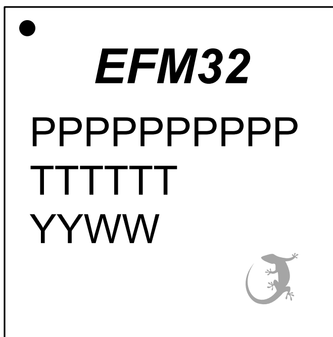
Figure 11.3. TQFP64 Package Marking
