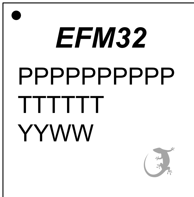
Figure 10.3. TQFP100 Package Marking
