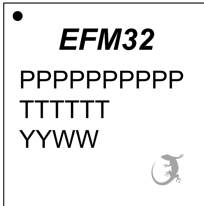
Figure 8.3. TQFP100 Package Marking
