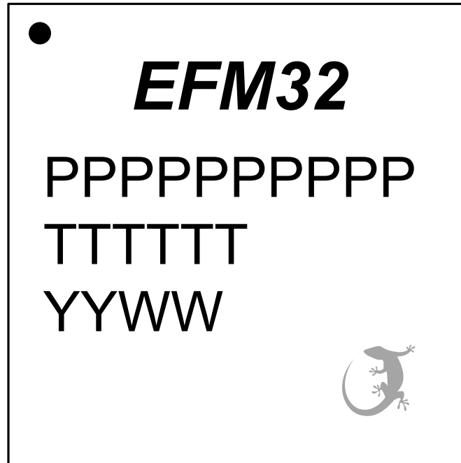
Figure 7.3. BGA112 Package Marking
