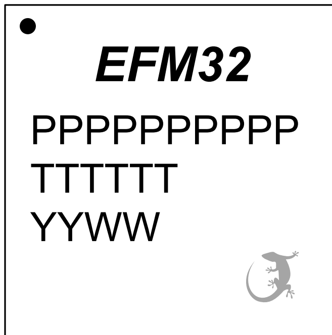
Figure 8.3. TQFP100 Package Marking
