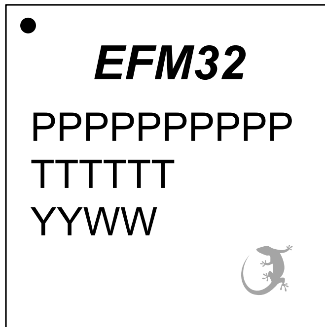
Figure 8.3. TQFP100 Package Marking
