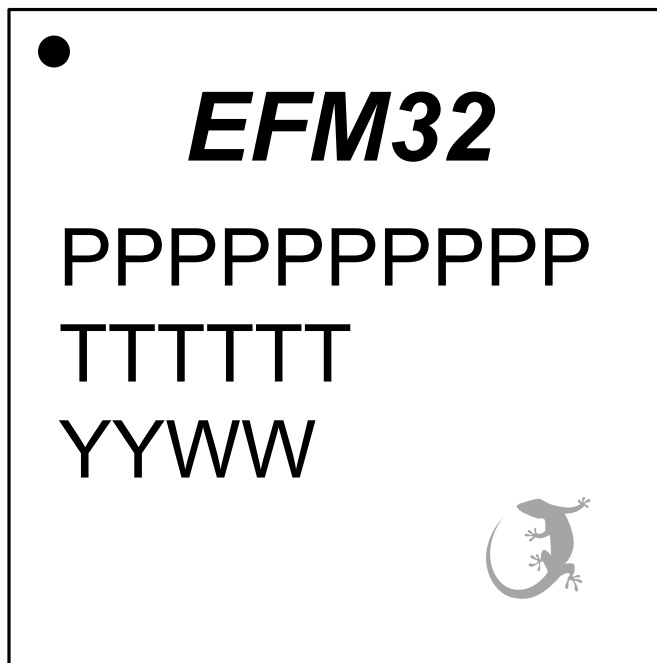
Figure 7.3. BGA112 Package Marking
