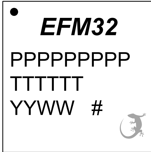
Figure 8.3. QFN32 Package Marking
