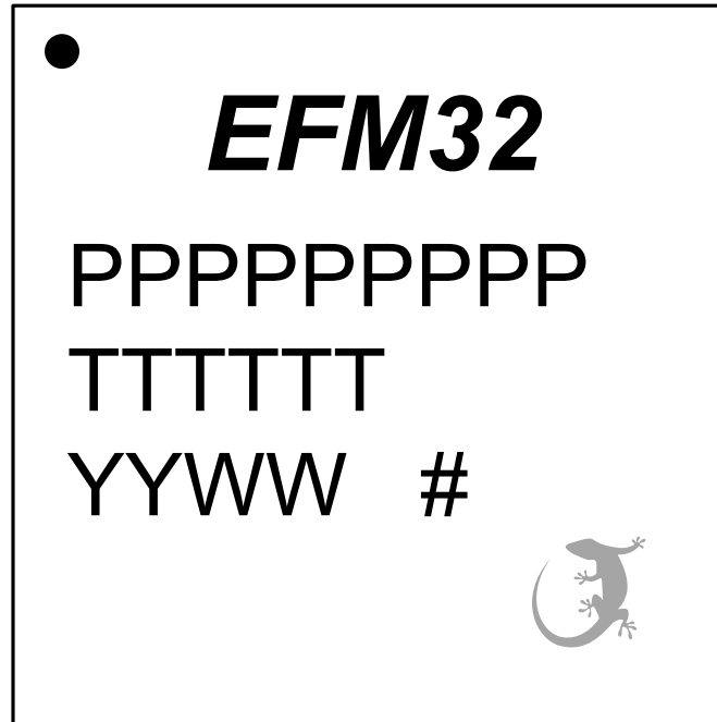
Figure 7.3. QFN48 Package Marking
