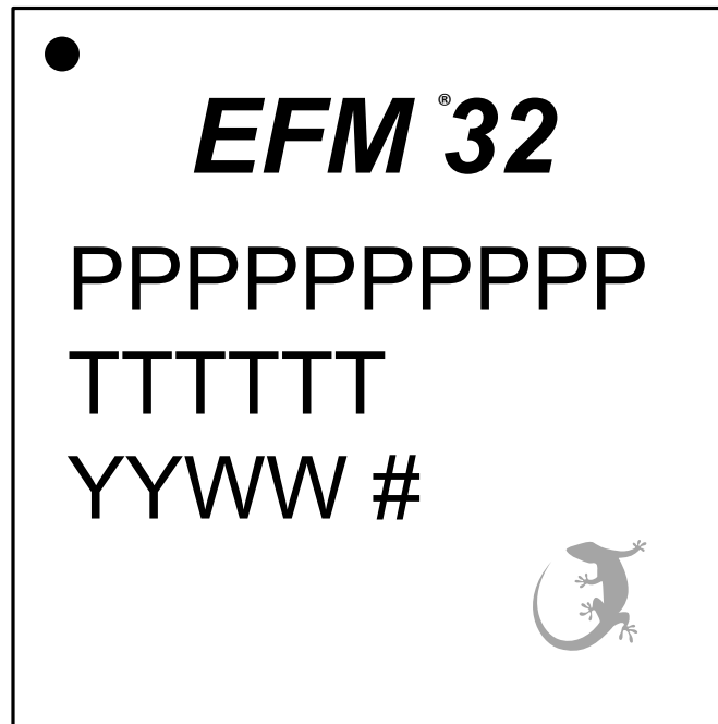
Figure 8.3. QFN48 Package Marking
