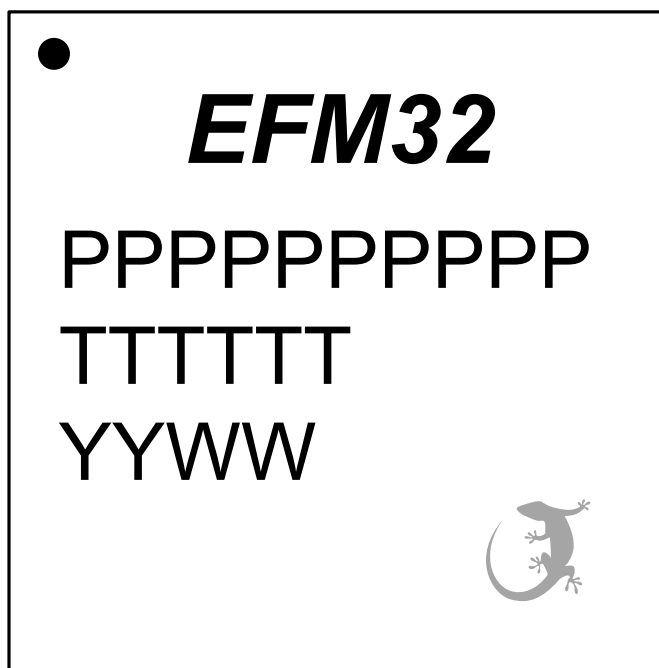
Figure 6.3. TQFP80 Package Marking
