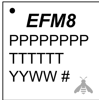
Figure 7.3. QFN28 Package Marking
