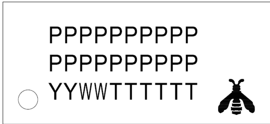
Figure 8.3. TSSOP28 Package Marking
