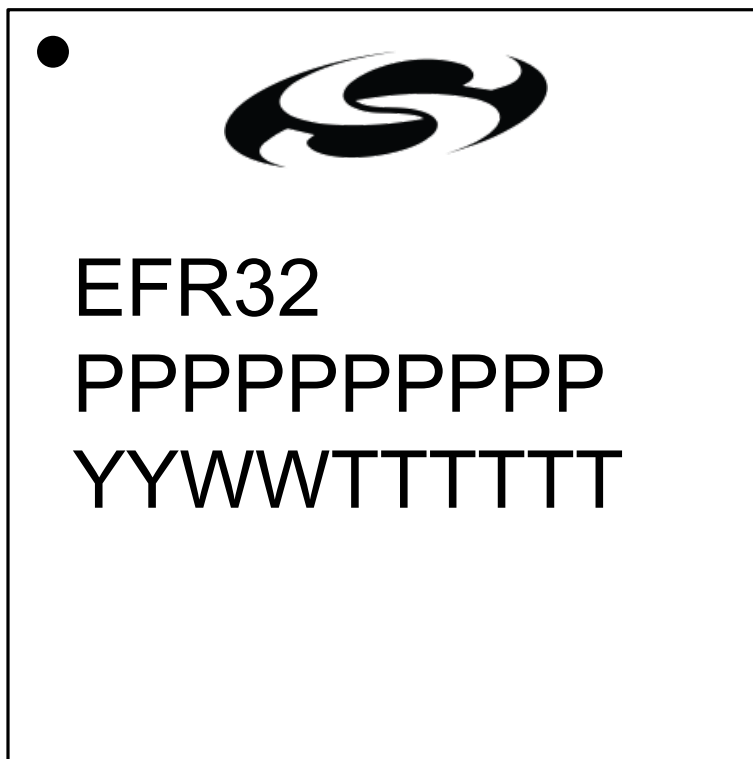
Figure 9.3. QFN68 Package Marking
