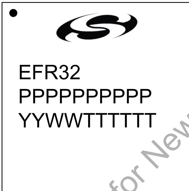
Figure 7.3. QFN48 Package Marking
