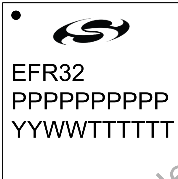
Figure 8.3. QFN32 Package Marking
