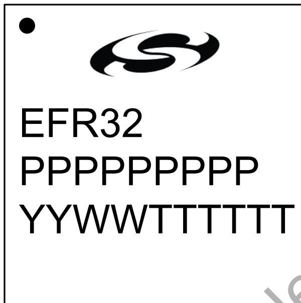
Figure 7.3. QFN32 Package Marking
