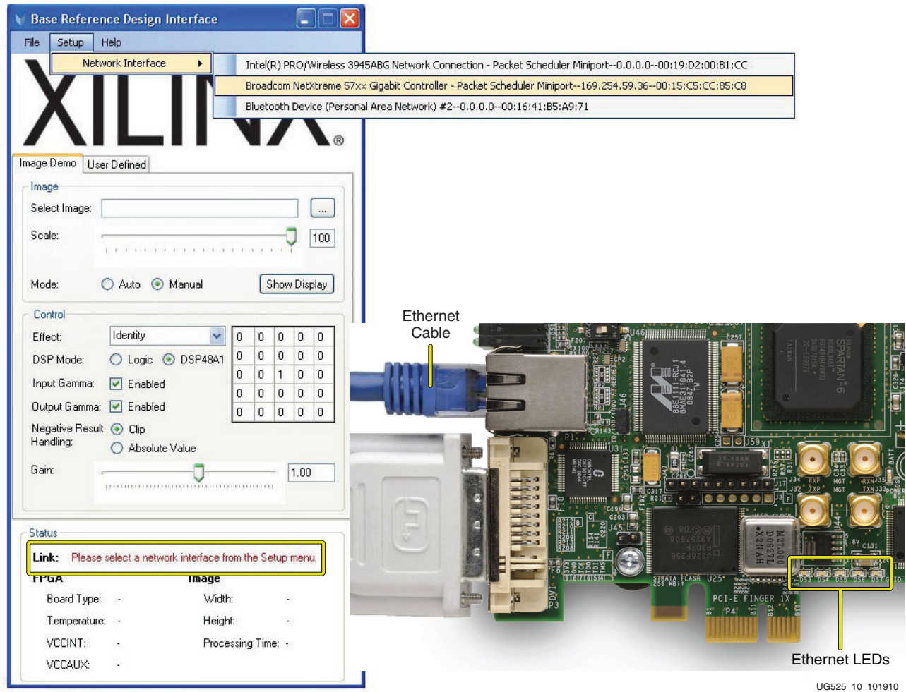
Figure 1-10: Connecting the Ethernet Link
