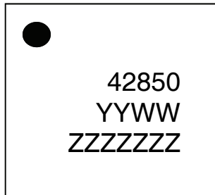
Figure 26. Top Marking Specification
