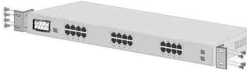
Figure 2.2: Attach mounting brackets with screws
