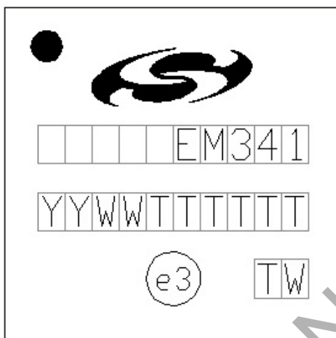
Figure 19.1. Part Marking for EM341
