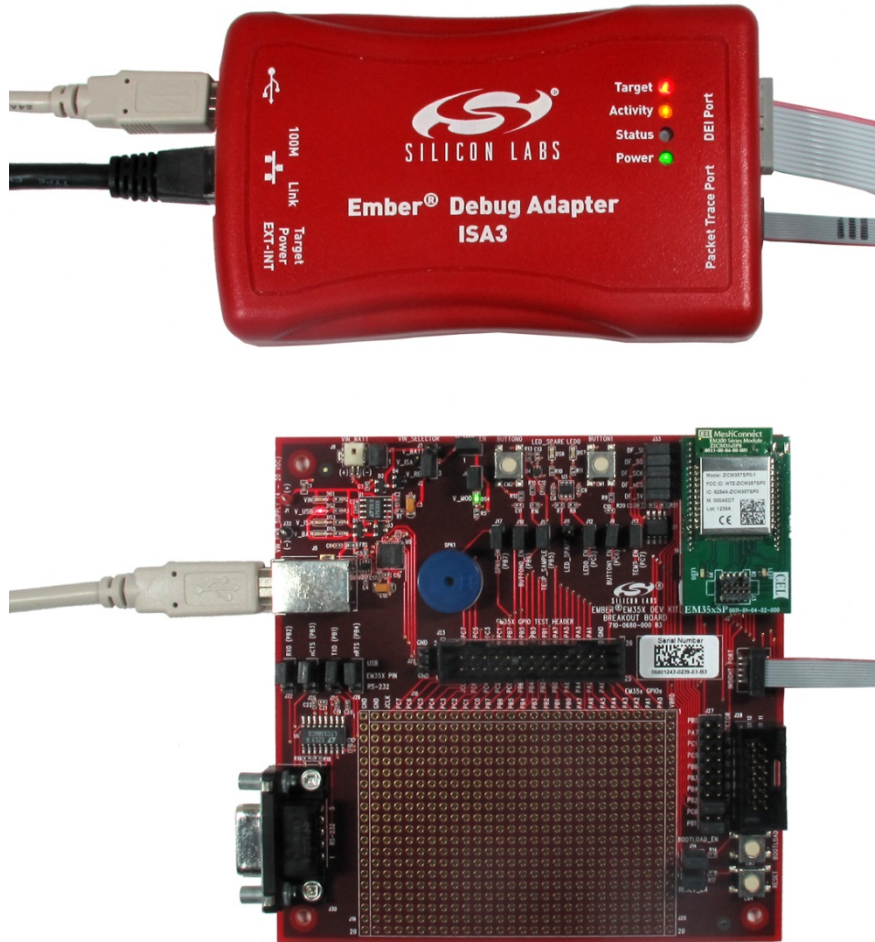
Figure 15. Ember Debug Adapter (ISA3) Supplying Power; FTDI Serial <-> USB Converter Used for Communication
