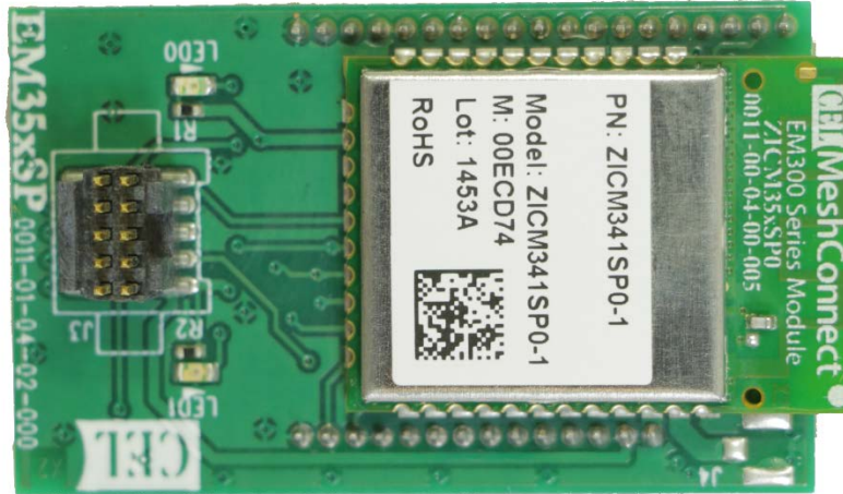
Figure 16. Module with PCB Antenna
