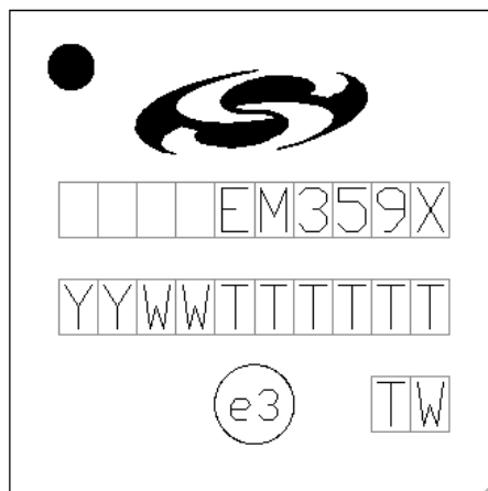
Figure 6.4. Part Marking for EM359x
