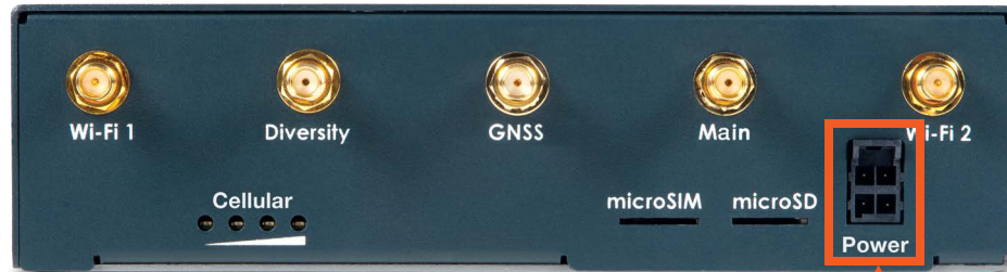
Figure 4-9 EMG 7500 Power Input
