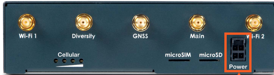
Figure 4-9 EMG 7500 Power Input
