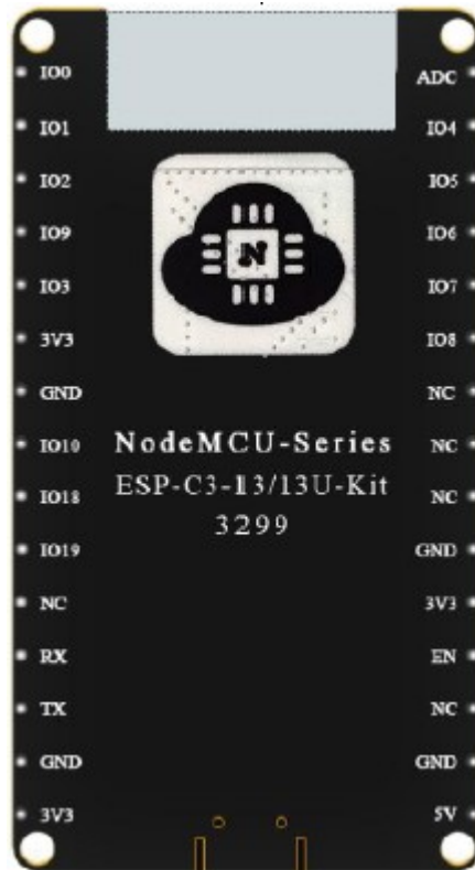
ESP-C3-13U-Kit Diagram of Pin
