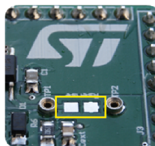
Figure 5. Pads for soldering SMD resistor
