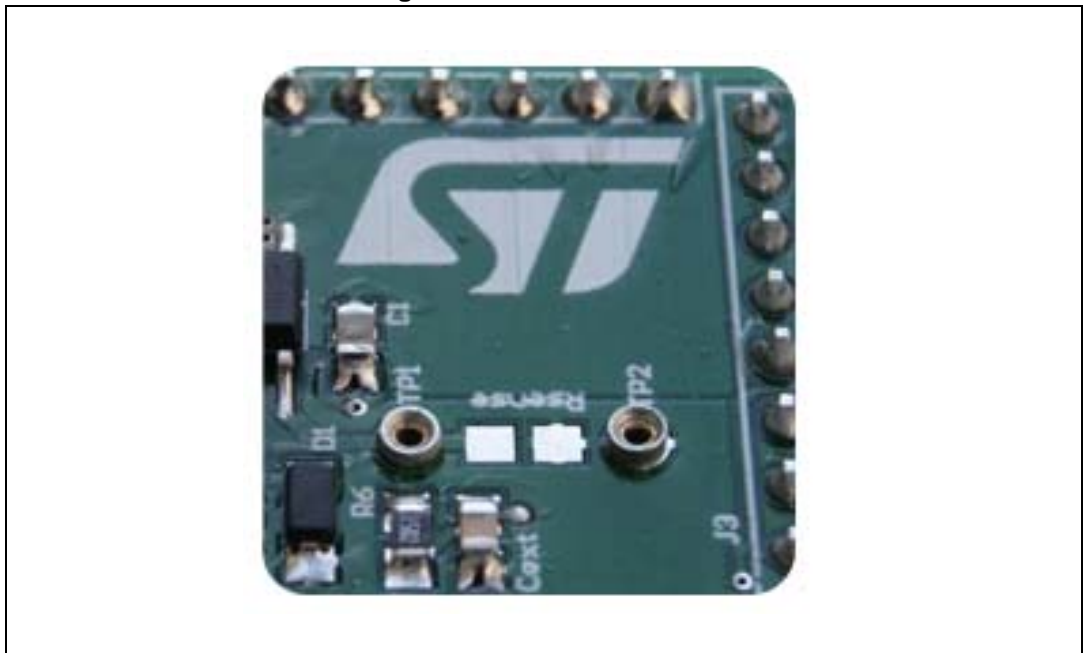
Figure 4. Mounting through-hole sense resistor
