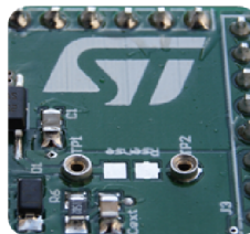
Figure 4. Mounting through-hole sense resistor
