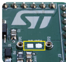
Figure 5. Pads for soldering SMD resistor
