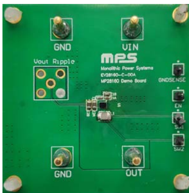
Total solution size (L x W) 6.9mm x 7.2mm
