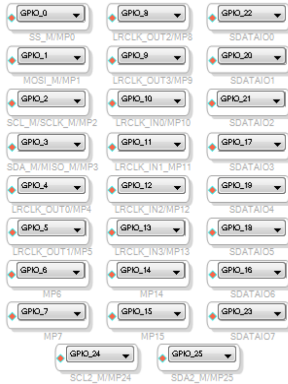
Figure 76. Complete Set of General-Purpose Outputs in SigmaStudio
