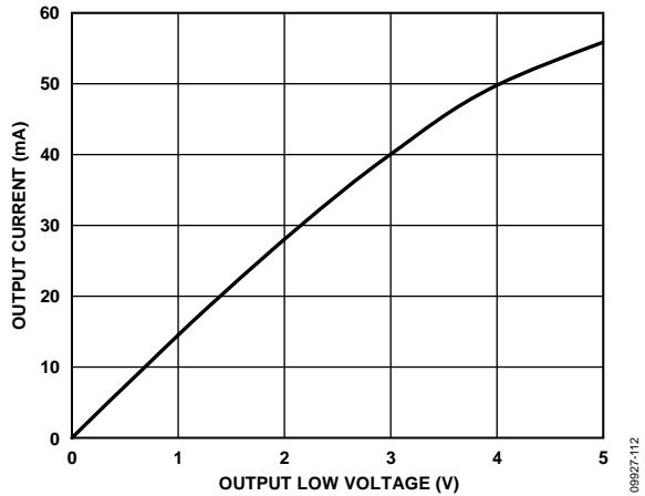
Figure 16. Receiver Output Current vs. Receiver Output Low Voltage
