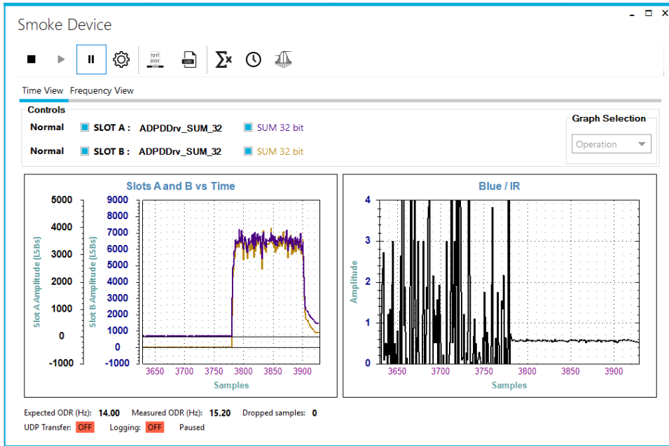
Figure 9. Raw Data and Ratio with Smoke Particles Present
