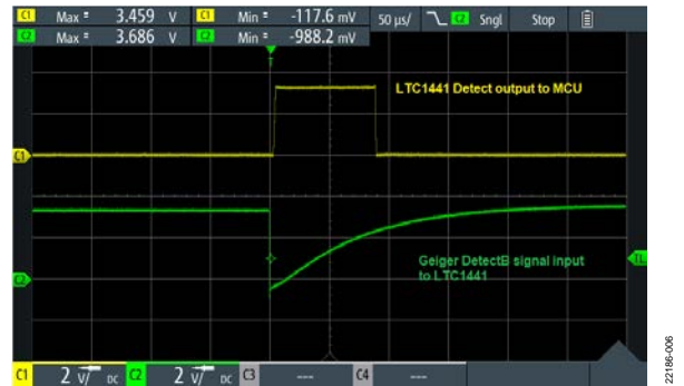
Figure 6. Geiger-Mueller Output Pulse Detection and LTC1441 Output Pulse
