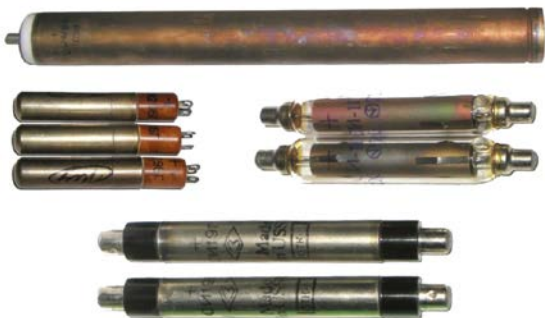
Figure 2. Geiger-Muller Sensor Tubes
