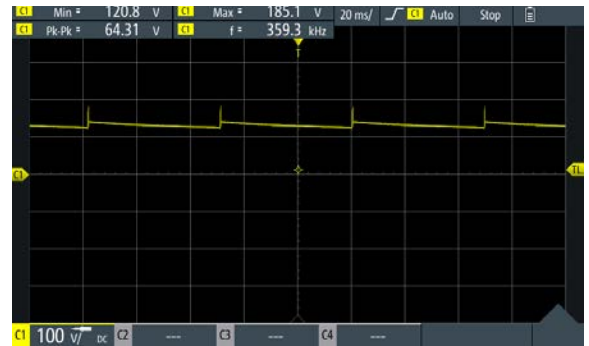
Figure 10. Hysteretic Regulation Measured at C11 at a Time Scale of 20 ms
