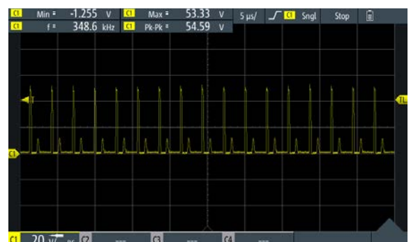
Figure 13. Boost Pulses at MOSFET Q2 Drain Terminal at a Time Scale of 5 \mu s
