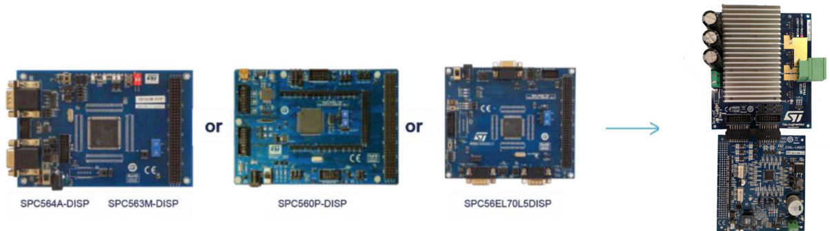
Figure 3. SPC56 discovery + application examples + EVAL-L9907-H
