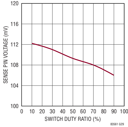
SENSE Current Limit vs Duty Ratio
