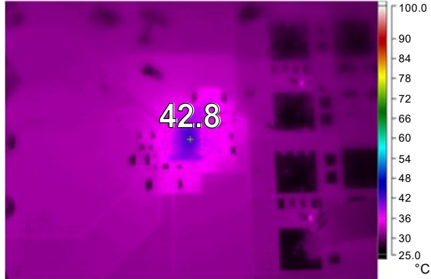
Figure 7. Thermal Picture at V CC = 10V, Both G1 and G2 are running at 2MHz, C LOAD = 3.3nF, no forced air flow
