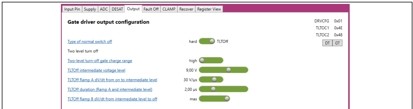
Figure 19 Output settings of the gate driver
