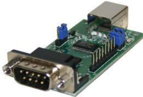
Figure 1.1 – EVAL232R FT232RL USB to RS232 Evaluation Module
