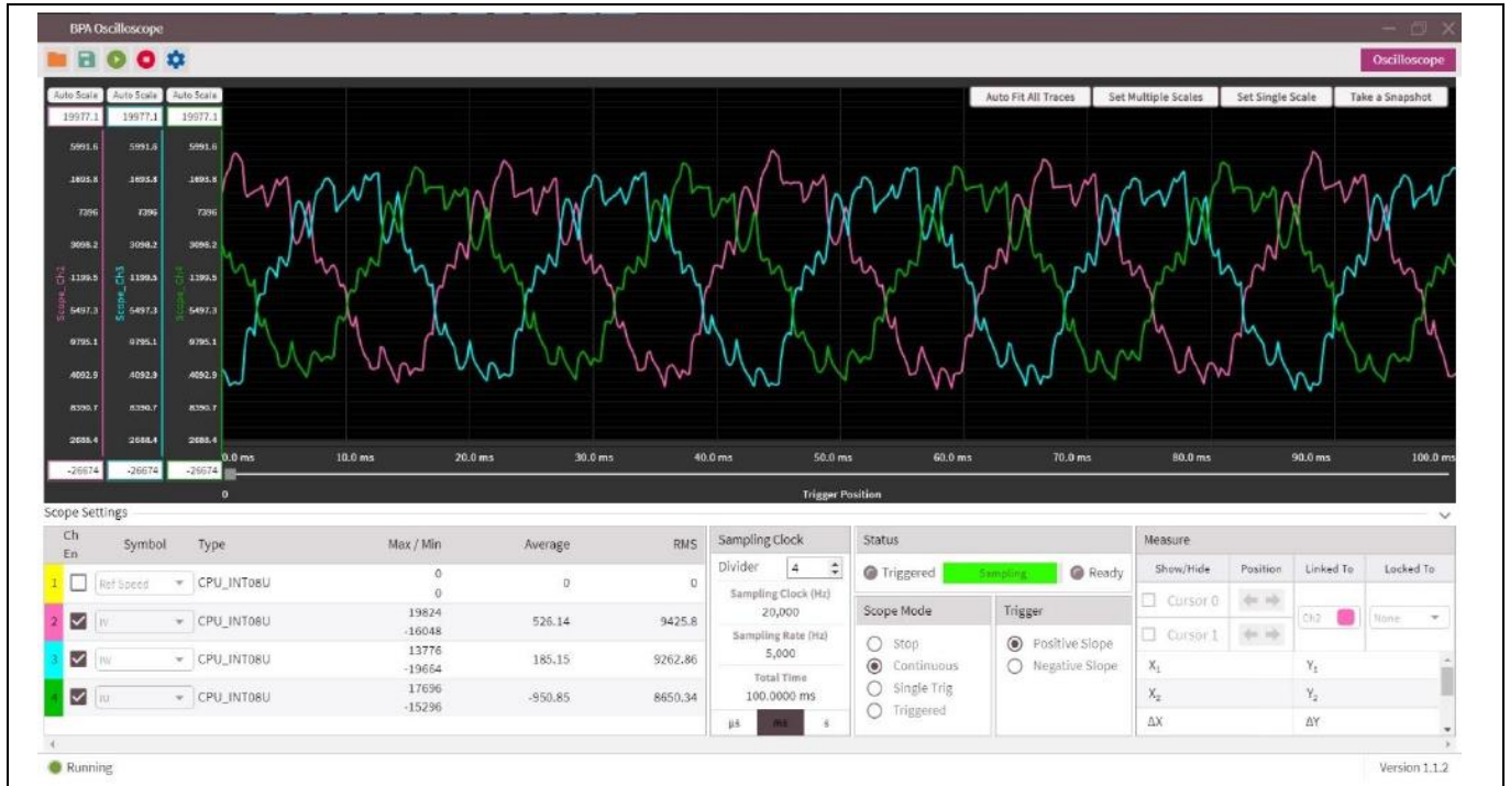
Figure 53 Oscilloscope view showing the phase currents; I_u (green), I_v (red), I_w (blue)
