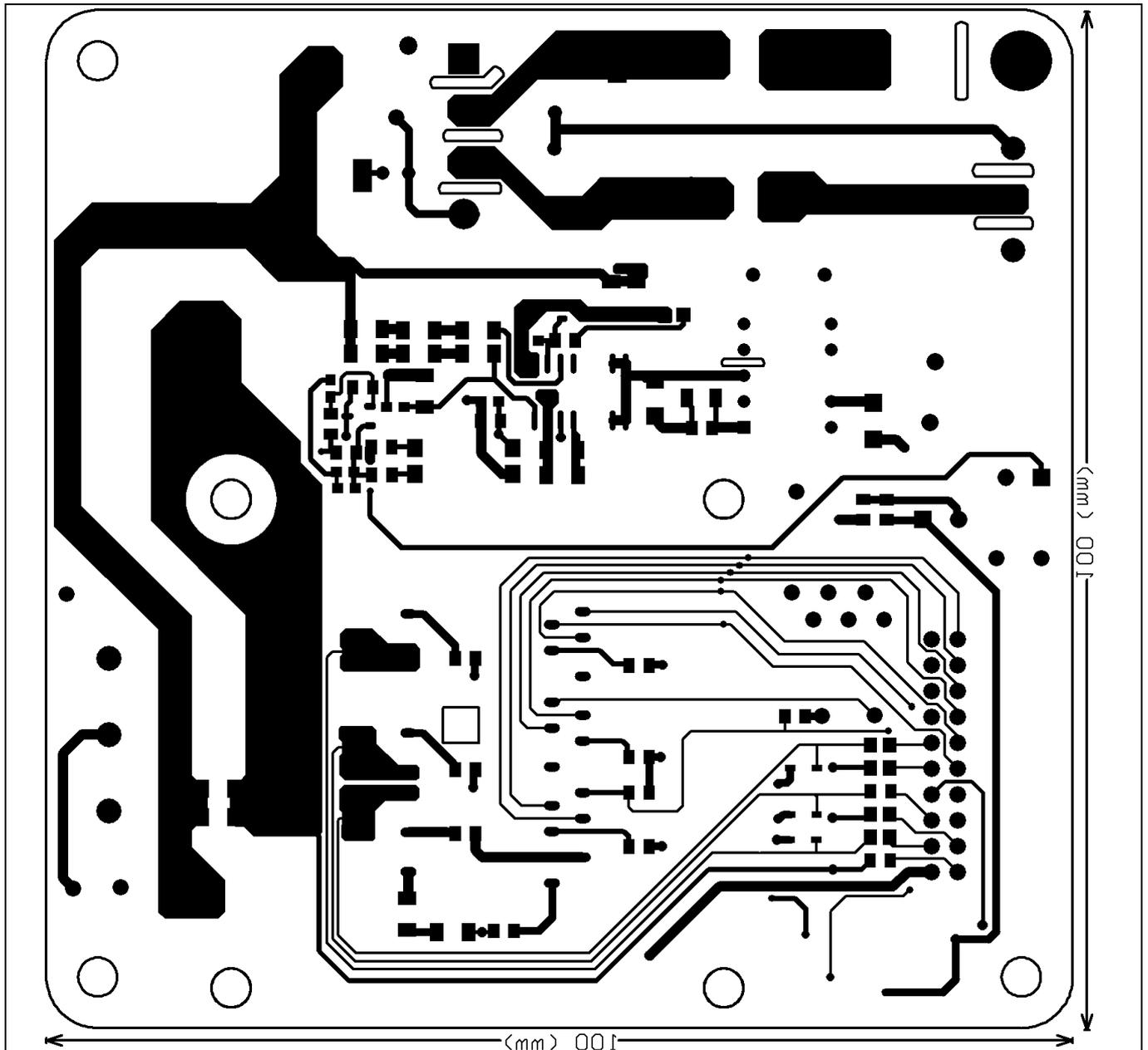
**Figure 26** Bottom layer routing of the EVAL-M1-IM231-A
