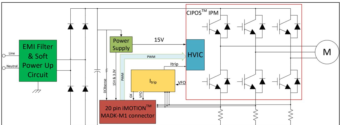
**Figure 1 The Block Diagram of the EVAL-M1-IM231-A Evaluation-board**
