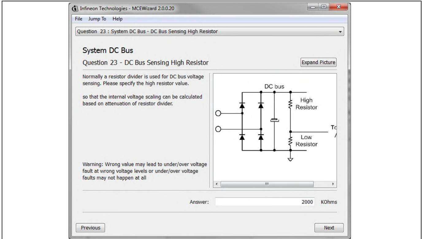
**Figure 11 DC bus sensing configuration in MCEWizard**
