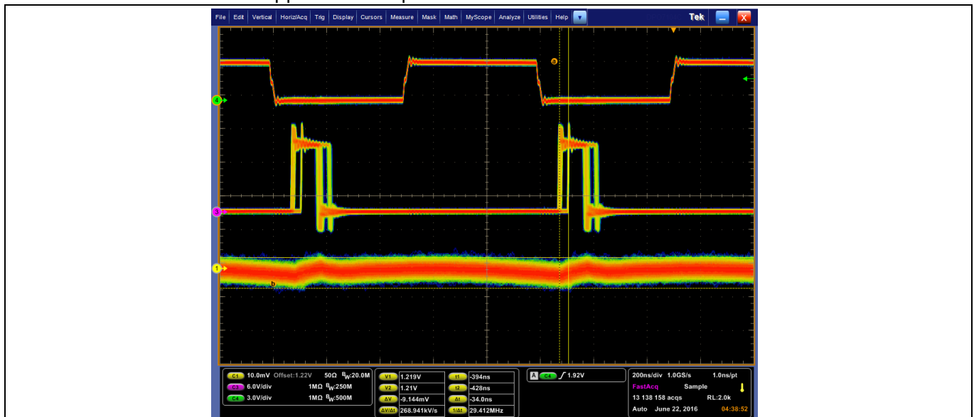
Figure 19 TOP→SYNC in, MIDDLE→SW_NODE, BOTTOM→RIPPLE
