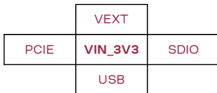
Figure 11: External power supply selection, J104-J106
