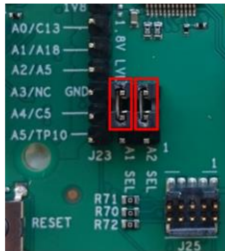
Figure 6: A1 and A2 as analog in on J2
