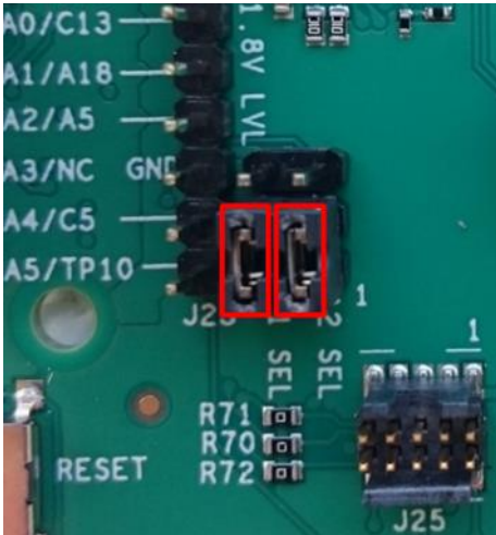
Figure 7: A1 and A2 as digital I/O on J2
