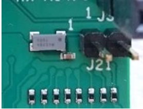
Figure 9: 32.768 kHz oscillator and pin header J21
