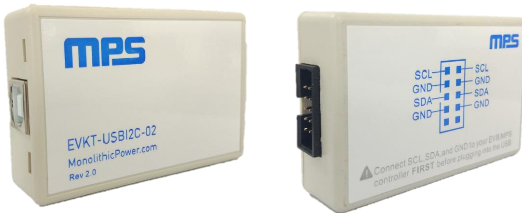
Figure 3: EVKT-USBI2C-02 Communication Interface Device
