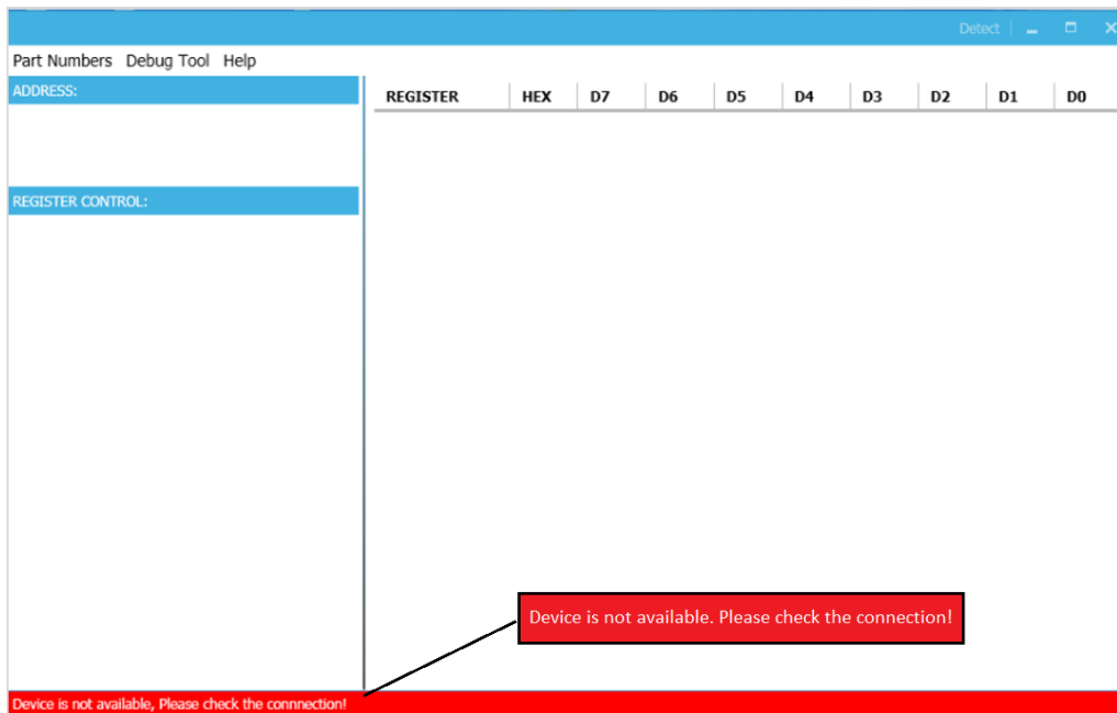
Figure 9: Warning Indicates Unsuccessful Connection – USBI2C Communication Interface Device is Not Connected
