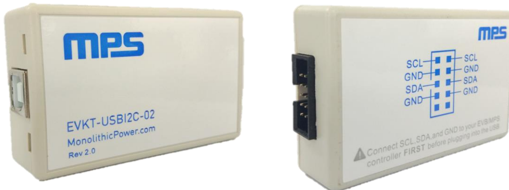
Figure 3: EVKT-USBI2C-02 Communication Interface
